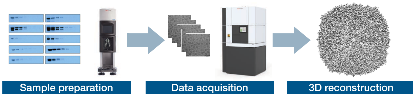
Figure 2. Schematic representation of the SPA workflow. After the biochemical steps of protein purification and verification, the samples are ready for cryo investigation. Cryo-grids are prepared using the Thermo Scientific Vitrobot™ System. Subsequently, they are transferred into the Glacios Cryo-TEM for sample optimization and high-resolution data acquisition followed by 3D reconstruction of the protein.
